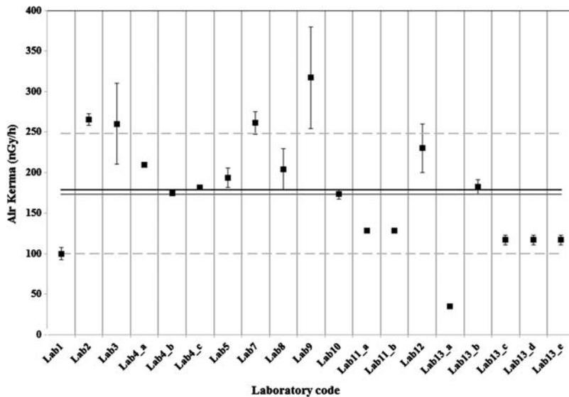
Figure 5. Results obtained at point X (uranium tailings). The grey line indicates the reference value by CIEMAT. The black line indicates the average of the participant mean values and the light grey dashed lines one standard deviation up and below the average value.
