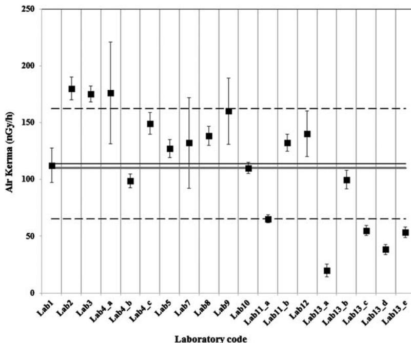
Figure 3. Results obtained at Station 1 (restored area). The grey line indicates the reference value by CIEMAT. The black line indicates the average of the participant mean values and the light grey dashed lines one standard deviation up and below the average value.
