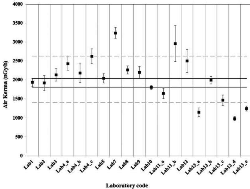
Figure 4. Results obtained at Station 2 (no restored uranium tailings area). The grey line indicates the reference value by CIEMAT. The black line indicates the average of the participant mean values and the light grey dashed lines one standard deviation up and below the average value.
